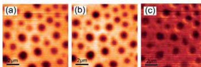
Conductive polymer film: X-ray microscopic image (STXM) showing two energy levels (a, b) and respectively calculated amount of solvent (dark = large amount of solvent) (c).
